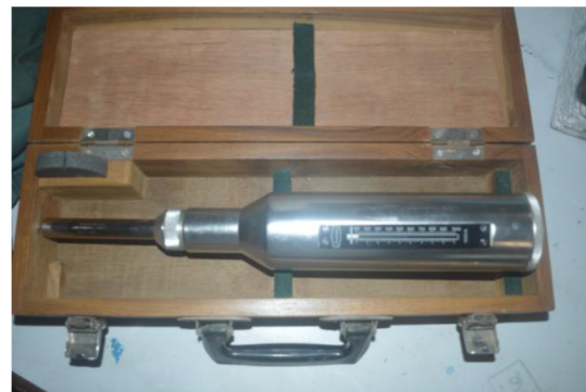
Figure 8: Non- Destructive Test using Schmidt Hammer
