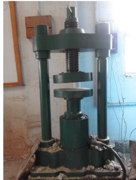
Figure 7: Destructive Test for compression strength Test
